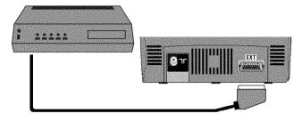
The respective scart socket is usually marked 'AV' or 'VCR' on the decoder or satellite receiver.
